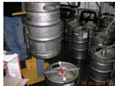
Double stacking kegs using the Keg Lifter and Stacksafe Base Support
